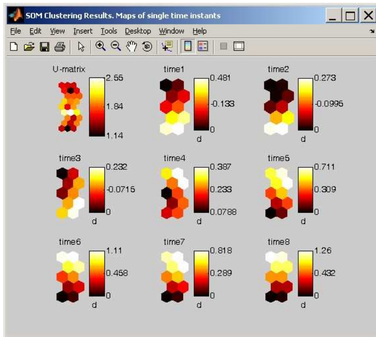
Figure 5: SOM results: the U-matrix and the maps of each time instant.
