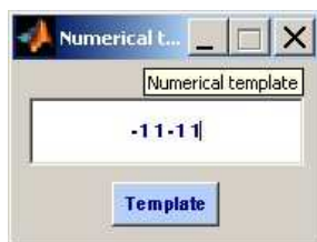
Figure 26: TAC. The window for the introduction of the label of the template to search. 1 indicates Increasing, 0 Steady and -1 Decreasing. Elements of the label are separated by white spaces.
