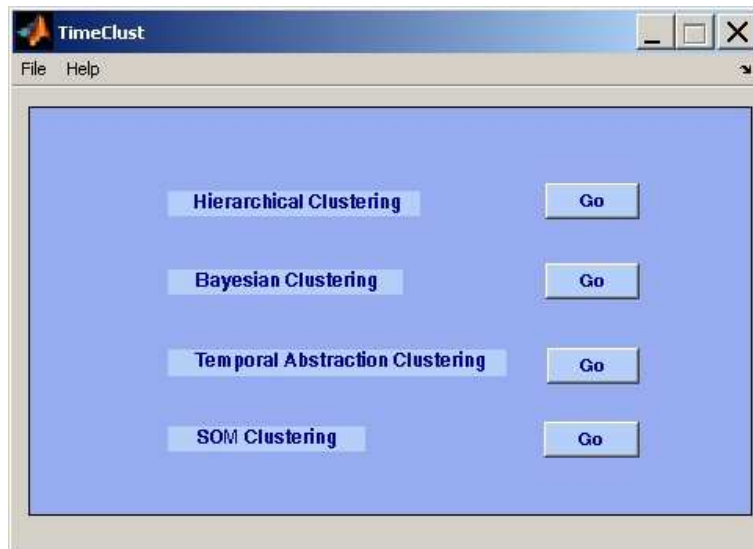
Figure 2: The TimeClust main window. Press one of the Go buttons to select the clustering algorithm.
